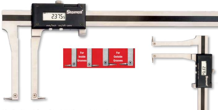
The 5006BZ-14/350 Electronic Groove Caliper is ideal for measuring internal and external grooves on large workpieces. This caliper is made of hardened stainless steel and is coolant resistant. With RS232 output, it is compatible with Starrett DataSure Wireless Data Collection Systems, which eliminates output cables.
